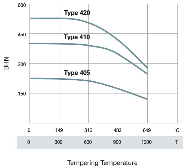
Carbon content is increased to a 0.15% minimum (0.30% nominal) compared to the 0.15% maximum limit for Type 410. Along with the carbon, chromium content is also slightly increased to offset the tendency of the higher carbon content to lower the alloy's resistance to corrosion.
