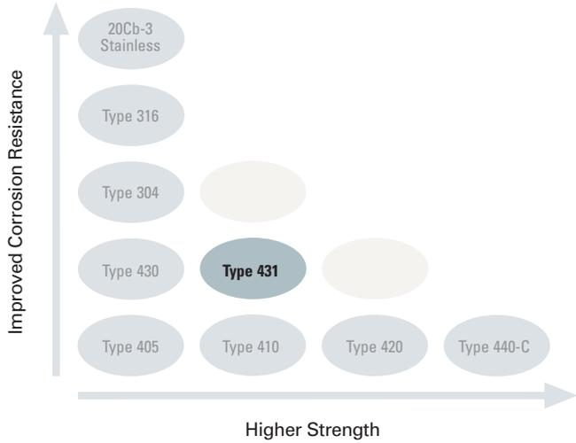
Type 431 is a magnetic, martensitic, stainless steel which is thermally hardenable. The carbon content is held between 0.12 and 0.17% compared to Type 430's maximum 0.12% carbon. With 1.50 to 2.50% nickel added, good toughness is maintained at high strength levels.
