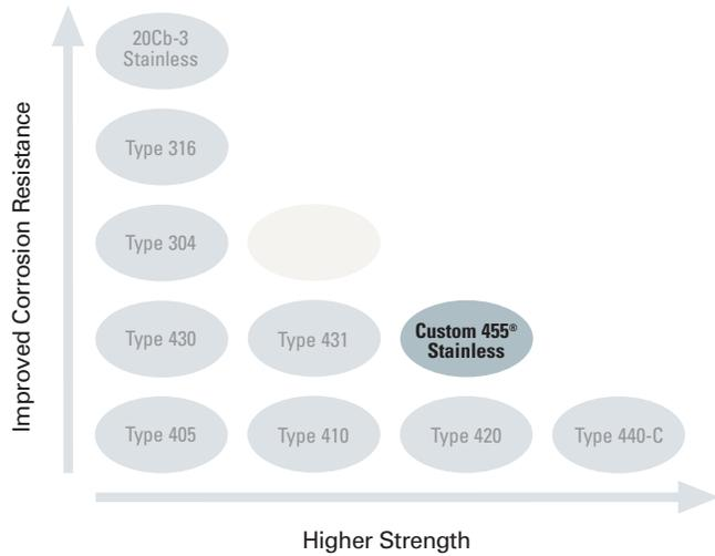
Custom 455 stainless may be classified as martensitic—age hardening or maraging. Unlike the preceding alloys, Custom 455 stainless is not strengthened by a simple carbon addition. Further additions of carbon would adversely affect its corrosion resistance and mechanical properties. Instead, Custom 455 stainless is strengthened by precipitation of a second phase, thereby achieving a special degree of corrosion resistance and strength.
