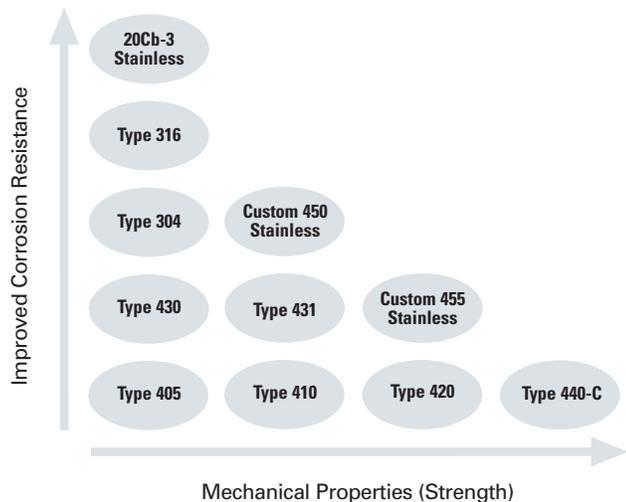
and 440-C differ in mechanical strength but have generally similar corrosion resistance.
