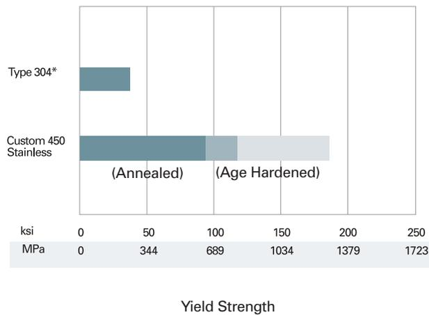
\* Note: Type 304 can be cold worked to higher strength levels, but only in small sections.
